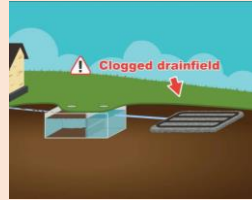
Standing water in the drain field/ leach field
