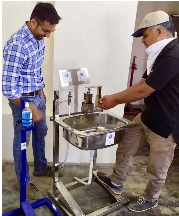
Low-cost portable foot-operated hand washing facility
