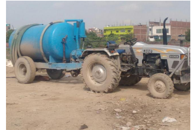
Tractor mounted (3,000 - 5,000 liters capacity)
