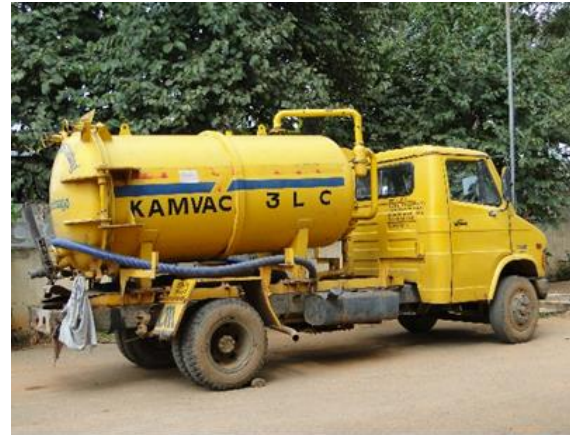
Truck mounted (1,500 - 10,000 liters capacity)
