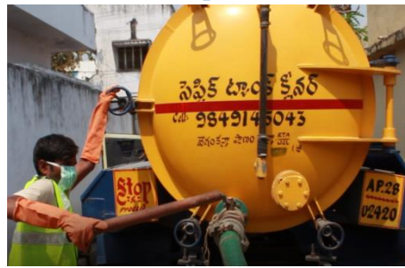
After the vacuum tank is full, close the valve
