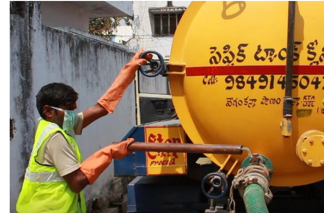
STEP 6: After the vacuum tank is full, close the valve
