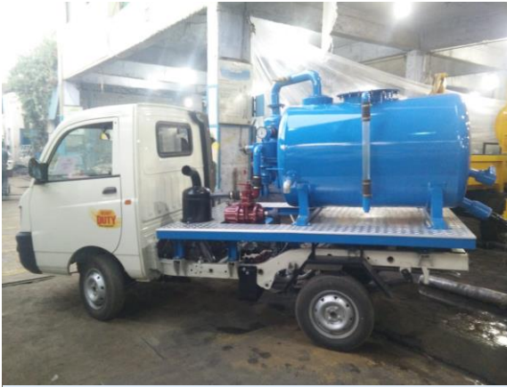
Truck mounted (500 - 800 liters capacity)
