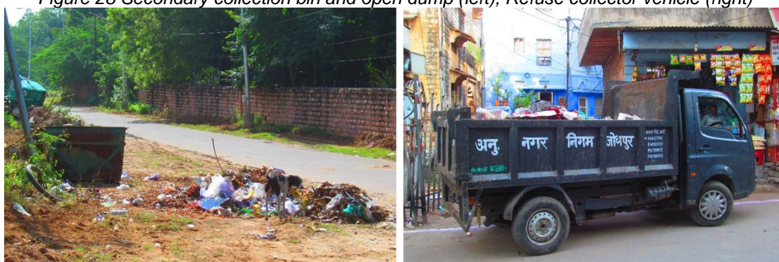
Figure 28 Secondary collection bin and open dump (left); Refuse collector vehicle (right)
