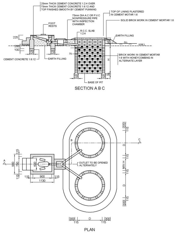
Figure 20 Twin pit in high subsoil water level
