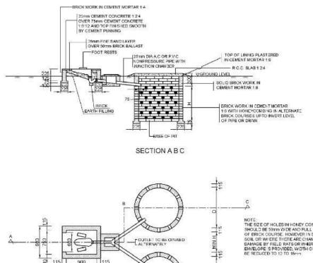
NOTE: THE SIZE OF HOLES IN HONEY COMBING SHOULD BE SOMM VIDE AND FULL HEIGHT OF BRICK CONTREL HONEVER IN SAMP SOIL OR WHERE THERE AND CHARGE OF DAMAGE BY FIELD RATS OR WHERE SAND ENVELOPE IS PROVIDED, WIDTH OF HOLES BE REDUCED TO 12 TO 15mm
