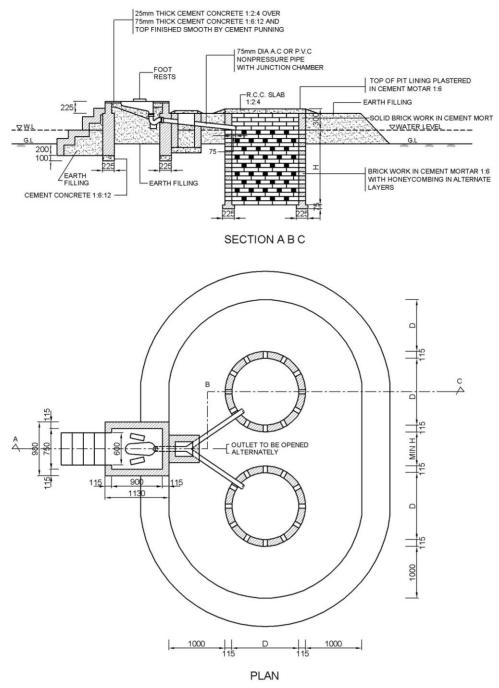
Figure 19 Twin pit for water logged area
