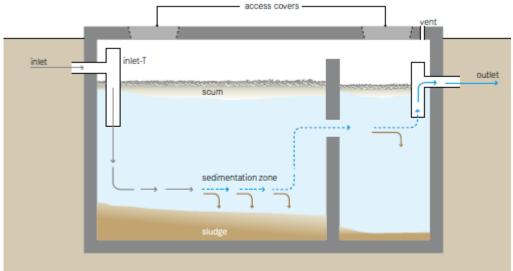
Figure 4 Double chambered septic tank
