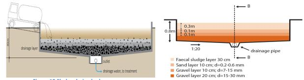
Figure 15 Sludge drying beds Image source: Compendium of Sanitation Systems and Technologies - 2nd Revised Edition and Advisory on septage management
