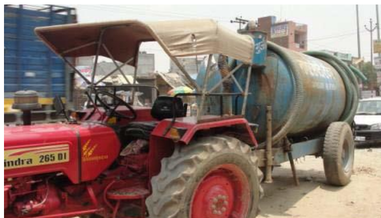
Figure 18 Septage emptying vehicle
