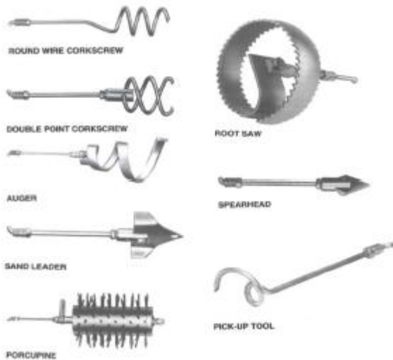
Figure 15 Rod heads for scraping septic tanks and sewer lines recommended by CPHEEO
